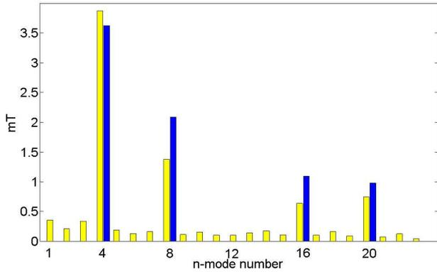
Fig.2: #20079  $m=0$  mode spectrum. Averaged amplitudes of harmonics in the time window of application of (0,4) mode: measured (light bars) and calculated (dark bars).
