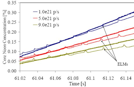
Figure 3: Neon concentration in the plasma core for three deuterium puffs levels,  $1 \times 10^{21}$  p/s;  $5 \times 10^{21}$  p/s and  $9 \times 10^{21}$  p/s and H-mode plasmas with (continuous line) and without ELMs (shaded line)
