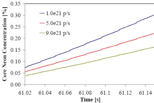
Figure 2: Neon concentration in the plasma core for three deuterium puffs levels,  $1 \times 10^{21}$  p/s;  $5 \times 10^{21}$  p/s and  $9 \times 10^{21}$  p/s and H-mode plasmas.
