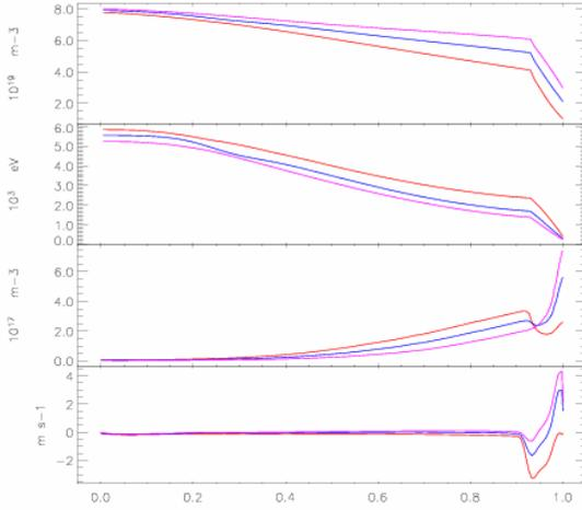
Figure 1: Plasma core profiles for three deuterium puffs levels,  $1 \times 10^{21}$  p/s (red);  $5 \times 10^{21}$  p/s (blue) and  $9 \times 10^{21}$  p/s (pink) of: a) ion density; b) ion temperature; c) total impurity and d) average over all ionisation stages impurity velocity.
