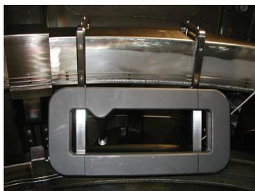
Fig.1. One coil of the TAE Antenna array on MAST
