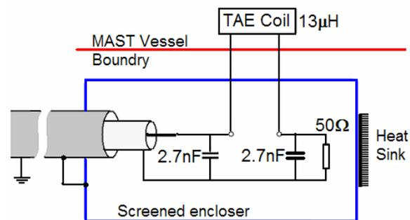
Figure 3: Schematic of the matching circuit used with TAE coil. The circuit is fitted in a screened enclosure mounted over the coaxial feed-through for the TAE coil.
