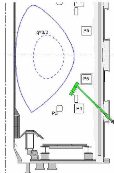
Figure 2: Position of the TAE antenna array w.r.t a typical MAST equilibrium. Pulse #10597,  $t=255\text{ms}$
