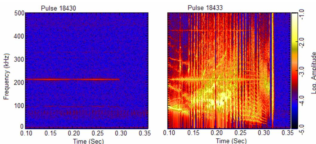
Figure 6: Spectral analysis of signal from Mirnov coil – OMAHA 5.2, for a pulse with (#18433) and without (#18430) plasma. Injection frequency 212kHz.
