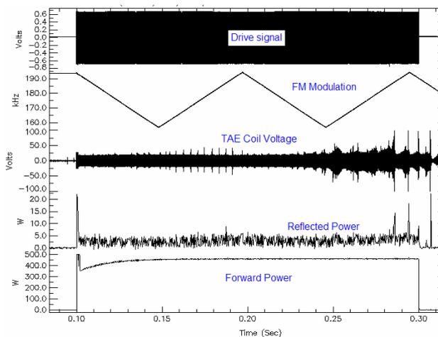
Figure 5. Signals from TAE coil and power supply monitoring diagnostics for pulse 18303.
