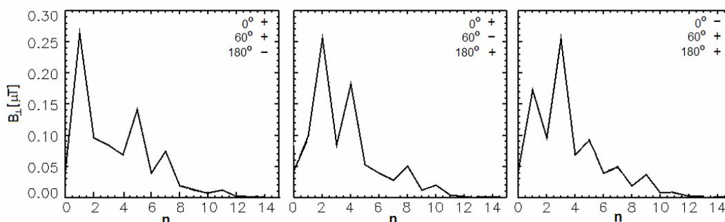
Figure 4: Amplitude of field perturbation calculated on the  $q=3/2$  surfaces for various combinations of currents in the MAST three coil TAE antenna array. Coil current 4A.turn. In the three cases shown the dominant perturbation is either  $n=1$ , 2, or 3.
