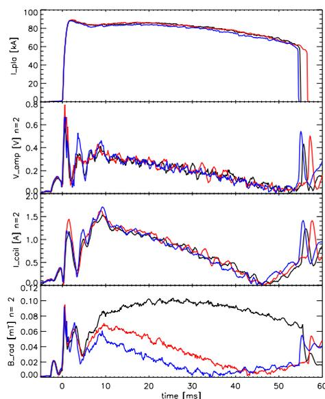
Figure 2. Intelligent shell feedback with PI-controller. From top: Plasma current,  $m=1, n=2$  Fourier amplitude of controller output voltage, coil current, sensor radial field. Discharges with fixed proportional feedback gain ( $K_p=80$ ) and varying integral gain:
