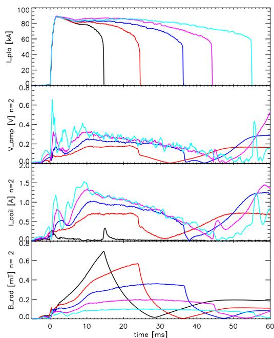
Figure 1. Intelligent shell feedback with P controller. From top: Plasma current,  $m=1, n=2$  Fourier amplitude of controller output voltage, coil current, sensor radial field. Discharges with varying proportional feedback gain: #20442: w/o fb (black) #20443:  $K_p=10$  (red) #20444:  $K_p=20$  (blue) #20445:  $K_p=40$  (magenta) #20446:  $K_p=80$  (cyan)
