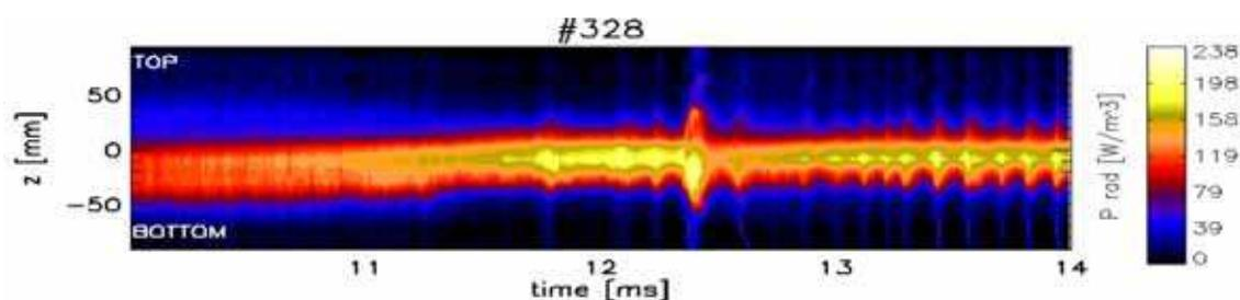
Fig.1a Radiated power detected by AXUV-based fast bolometric array
