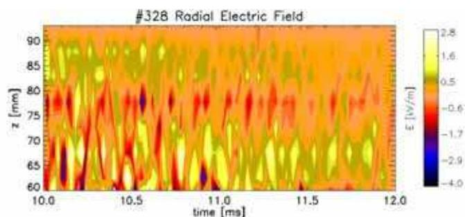
Fig 4 Local values of the radial electric field,  $E_{rad}$  deduced from the measurements of floating potential,  $U_{float}$
