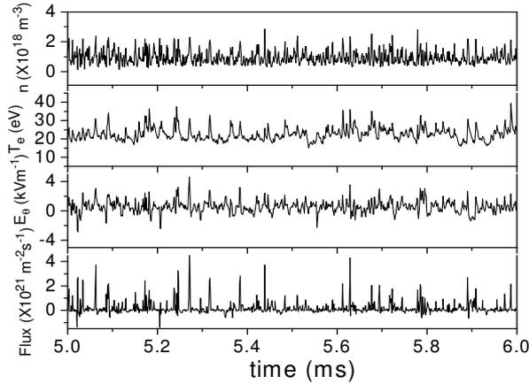
Fig.1. Time behaviours of the plasma parameters in the SOL: (from the top)  $n$ ,  $T_e$ ,  $E_\theta$  and  $\Gamma_r$ .
