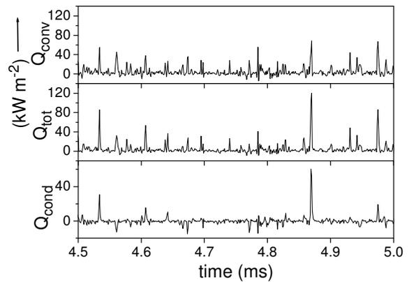
Fig. 4. Time dependences of (from the top) convected, total and conducted heat flux at  $r = 6.5$  cm.
