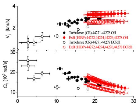
**Fig. 4.** Comparison of rotation velocities of density perturbations (black) with core plasma rotation (red) in OH (filled) and ECRH (open) plasma.
