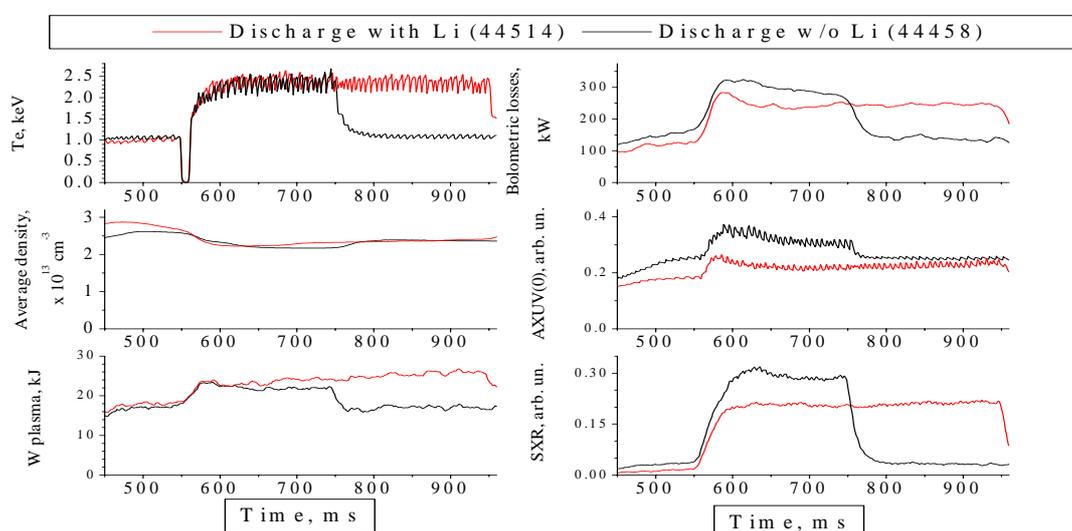
Figure 4. ECRH discharges characteristics with and without Li (short pulse-200 ms)
