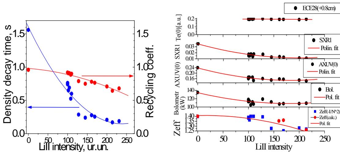
Figure 2. Recycling versus Li line intensity Figure 3. Discharge parameters versus Li deposit
