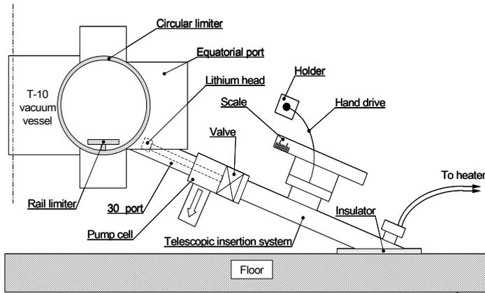
Two techniques of Li gettering were used. In the first one the Li-element was positioned in T-10 chamber before plasma experiments and heated up to the 450° C during two hours. The Li deposition to the chamber was about 20mg.
