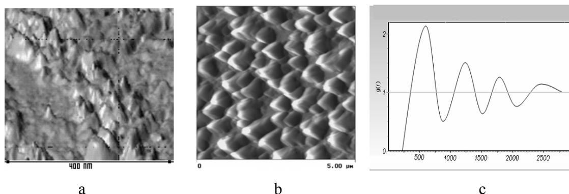
Figure 1. AFM image of deposited films after 10-th shot in T-10 2000 (a), after 30-th shot 2005 (b). Pair correlation function (c) for (b) structure.
