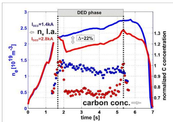
Figure 1: Electron density and normalized carbon concentration at center for discharge with low (blue) and high  $I_{\text{DED}}$  (red)
