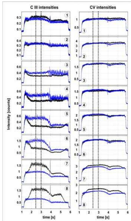
Figure 3: Time traces of CIII and CV line intensities for discharge w/o DED (blue) and with low DED
