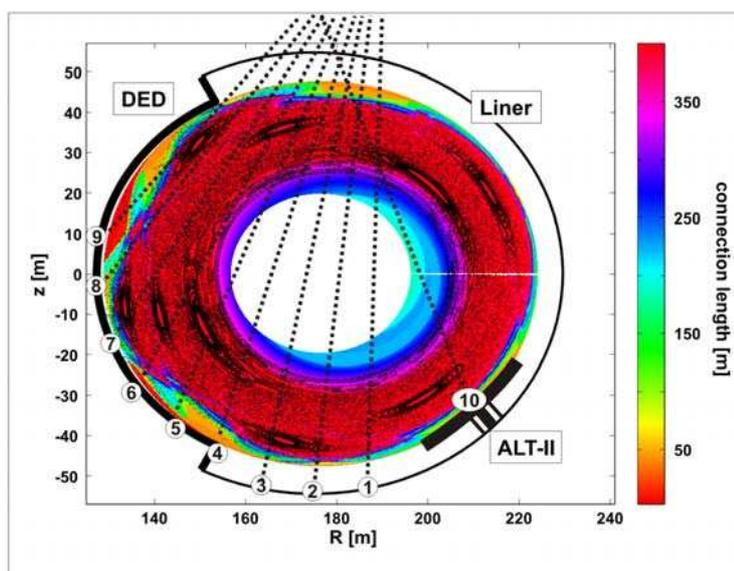
Figure 2: Magnetic field topology for #103900 ( $I_{\text{DED}}=2.8$ kA) with particle PO; superimposed are the lines of sight of the carbon spectroscopy system
