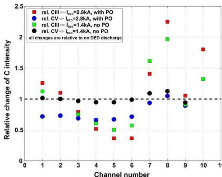
Figure 4: Change of CIII and CV intensities relative to no-DED discharge averaged for  $2.5s < t < 3.0s$
