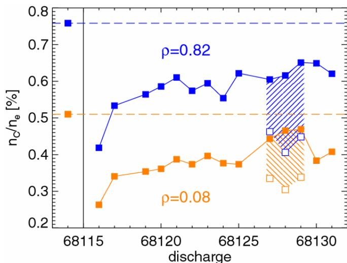
Figure 4: Evolution of carbon plasma concentration  $f_C = n_C/n_e$  in plasma centre (normalised radius  $\rho=0.08$ ) and outer plasma region ( $\rho=0.82$ ). The hatched areas denote the effect of a 6 cm plasma shift towards the central wall.
