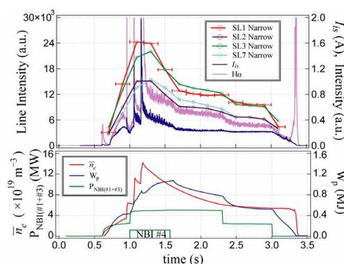
**Figure 4.** Time evolutions of line intensity of narrow component for several sight lines, the ion saturation current, line-averaged density, stored energy and the injected power with NB in a  $R_{ax}=3.6$ m configuration with pellet injections.
