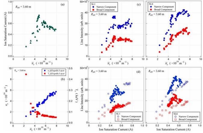
**Figure 3.**  $\bar{n}_e$  dependences of (a) ion saturation current, (b)  $n_e$  and  $T_e$  of edge plasma region and (c) line intensities at SL1 and SL6. (d) Line intensities are also plotted against ion saturation current.
