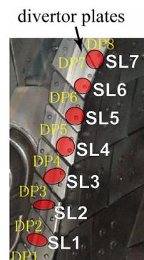
**Figure 1.** Spot positions of sight lines for observation of inboard divertor region.
