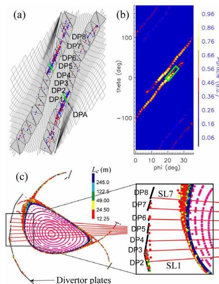
**Figure 2.** (a) Footprint of divertor field lines on the inboard divertor. The blue dots indicate the field lines with long connection length ( $L_c > 250$  m). (b) Particle deposition profile calculated with EMC3-EIRENE and (c) Poincaré plots of the field lines on observed cross-section.
