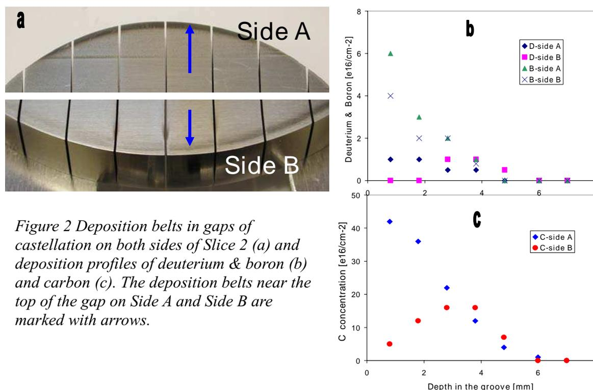
Figure 2 Deposition belts in gaps of castellation on both sides of Slice 2 (a) and deposition profiles of deuterium & boron (b) and carbon (c). The deposition belts near the top of the gap on Side A and Side B are marked with arrows.
