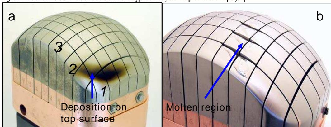
Figure 1. W macro-brush limiter after the first (a) and second (b) exposure at TEXTOR. Slices analysed with IBA are numbered 1-3.
