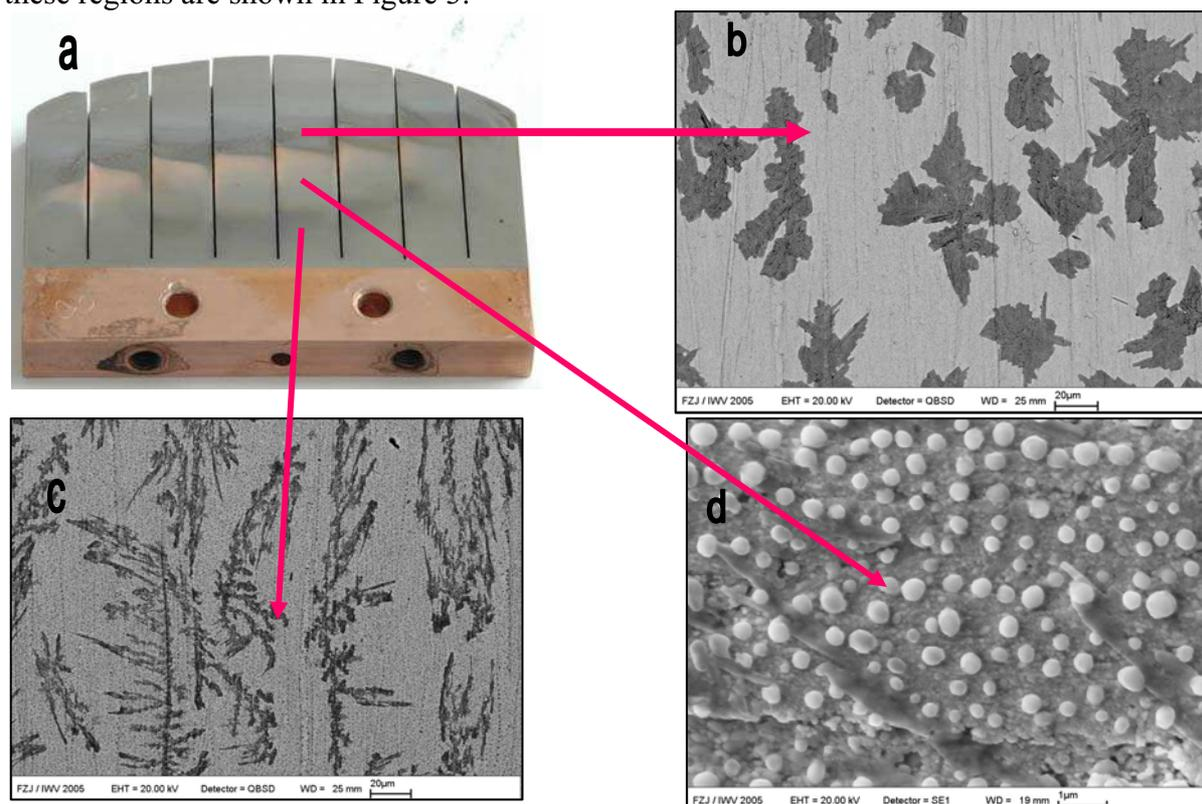
Figure 3. Overview (a) and SEM images of deposits structure in the poloidal gap (b) – (d).
