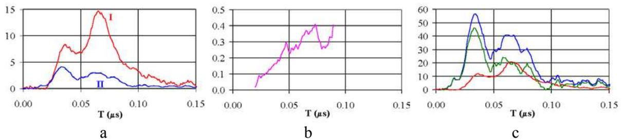
**Fig.5.** a) pin-diodes signals: I – filter 8μm Al, II – 0.25 μm Ag ; b) signals ratio taking into account the condition of registration; c) “recalculated” signals: — Al 8 μm ; — Ag 0.25 μm; — signals difference. P=1 Torr of neon, W=160 kJ
