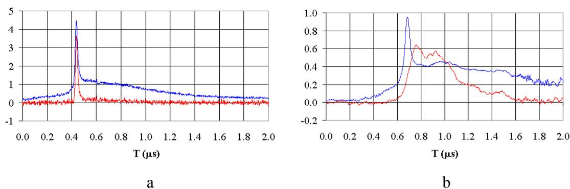
**Fig.6.** Pin-diode signals, filters Al  $8 \mu\text{m}$  (red beam) and  $0.25 \mu\text{m}$  Ag (blue beam): a) without liner,  $P=3$  Torr,  $W=645$  kJ); b) foam liner  $0.6 \text{ mg/cm}$ ,  $P=3.5$  Torr,  $W=645$  kJ
