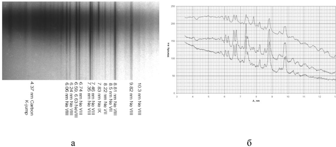
**Fig.4.** Spectrogram obtained for 6 shots at P=1 Torr and the spectrograph disposition at 60° to the system axis (a) и densitogram of this spectrum (b); the upper, middle and lower curves show a spectrum on distances 0; 4.5 and 9 mm from the pinch axis, respectively.
