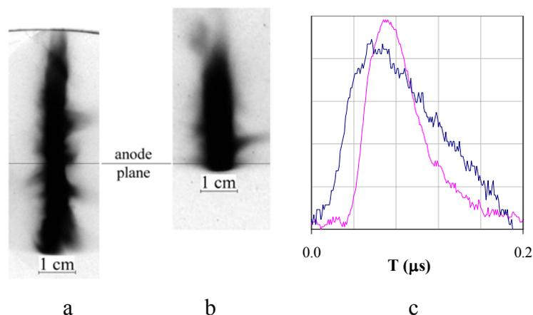
**Fig. 2.** Pin-hole pictures of the discharge in neon,  $W=540$  kJ,  $P = 1$  Torr: a) port 8 ( $60^\circ$ ), diaphragm 0.2 mm, filter Be 17 micron; b) port 6 ( $90^\circ$ ), diaphragm 0.4 mm, filter Be 10  $\mu\text{m}$  and pin-diode signals (c): red beam –detector D2 ( $90^\circ$ ), blue beam –detector D5 ( $60^\circ$ ), filter Al 8  $\mu\text{m}$
