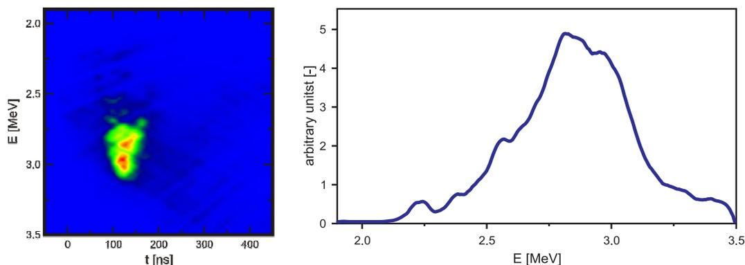
Fig. 2: Reconstructed time resolved energy spectrum (shot #6540, 24<sup>th</sup> October 2006) in downstream direction (left). The time integrated neutron energy spectra (right).
