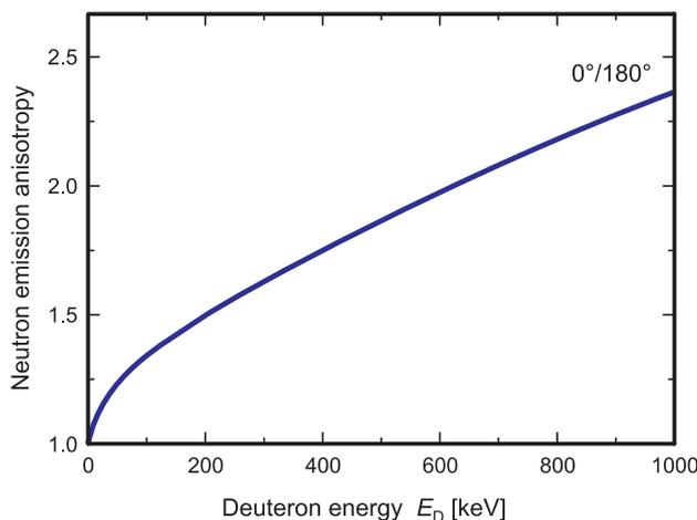
Fig. 1: The ratio between differential cross-section for  $\mathcal{A}_{LS} = 0^\circ$  and  $\mathcal{A}_{LS} = 180^\circ$  as a function of deuteron energy for D-D reaction. The angle  $\mathcal{A}_{LS}$  is the angle in the LS between fast deuteron and an emitted neutron.
