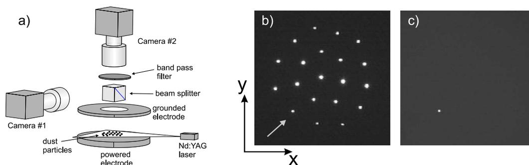
Figure 1: a) Scheme of the experimental setup. One of the trapped dust particles is the fluorescent tracer particle. See text for details. b) and c) Snap short of the dust cloud. (b) Image of camera #1 with all particles and (c) image of camera #2 that only sees the fluorescent tracer particle. In (b) the position of the tracer is marked by the arrow.
