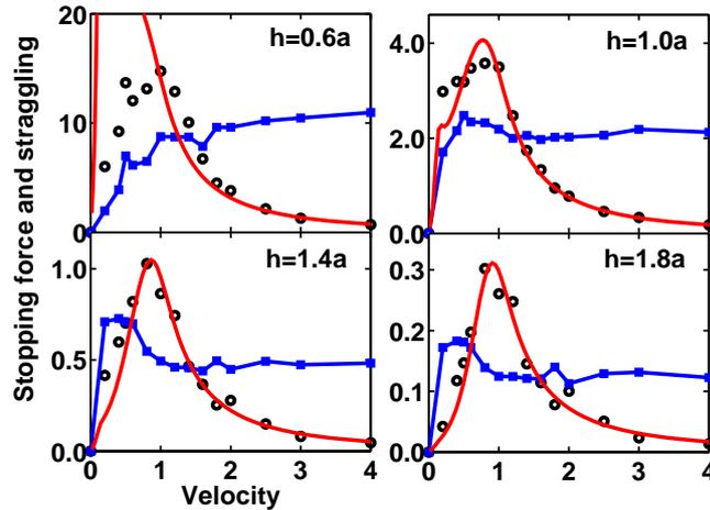
Figure 4: The (normalized) stopping force  $S$  versus the speed  $v_t$ , when  $\Gamma = 1000$  and  $\kappa = 1.0$ . Red solid lines and black circles are stopping forces from QLCA and BD, while the blue lines are their straggling from BD
