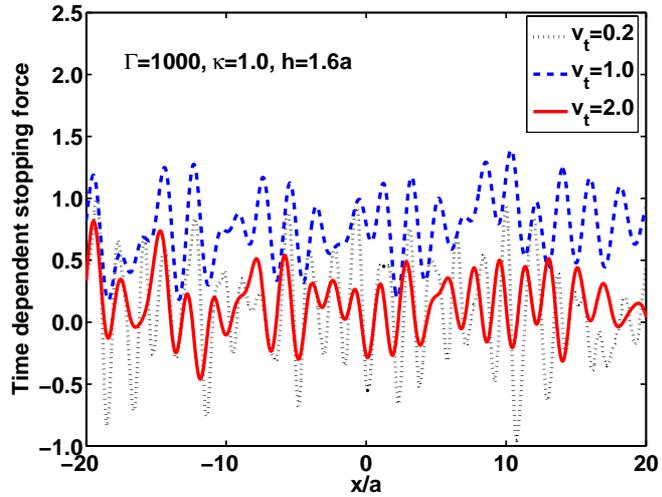
Figure 2: Time (position) dependent of the stopping force on the test particle
