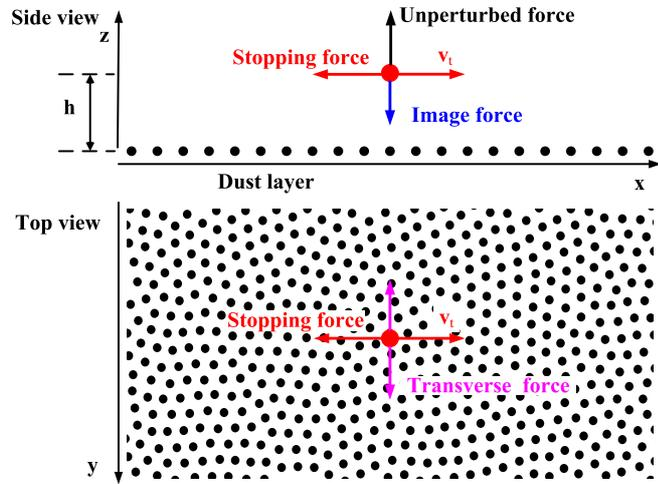
Figure 1: Schematic diagram for the model system and the definitions of the stopping force and image force
