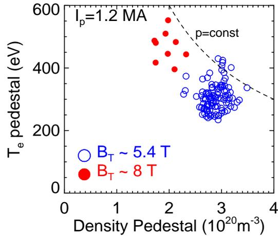
Figure 1. Pedestal  $T_e$  vs  $n_e$  for a set of 1.2 MA discharges at 5.4 T (blue) vs 7.9 T (red)
