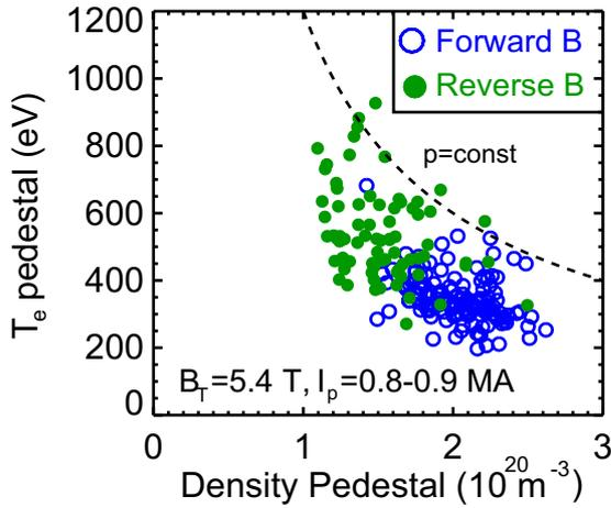
Figure 2: Pedestal  $T_e$  vs  $n_e$  for a set of 5.4 LSN discharges with forward  $B_T$ , 0.9 MA (blue) vs reversed  $B_T$ , 0.8 MA (green).
