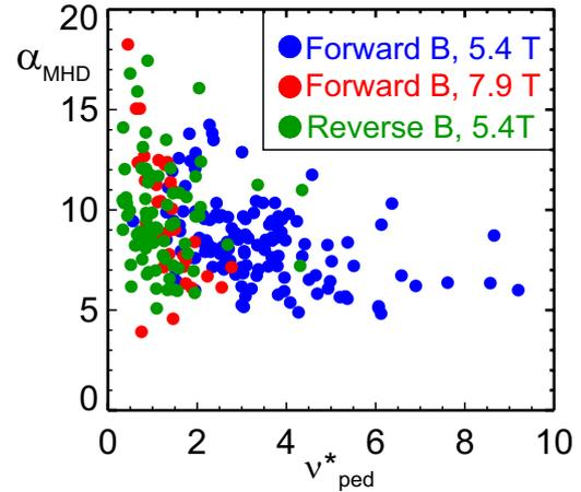
Figure 3:  $\alpha_{MHD}$  at the pedestal midpoint vs  $v^*_{ped}$  for forward field (blue 5.4 T, red 7.9 T) vs reversed field 5.4 T (green).
