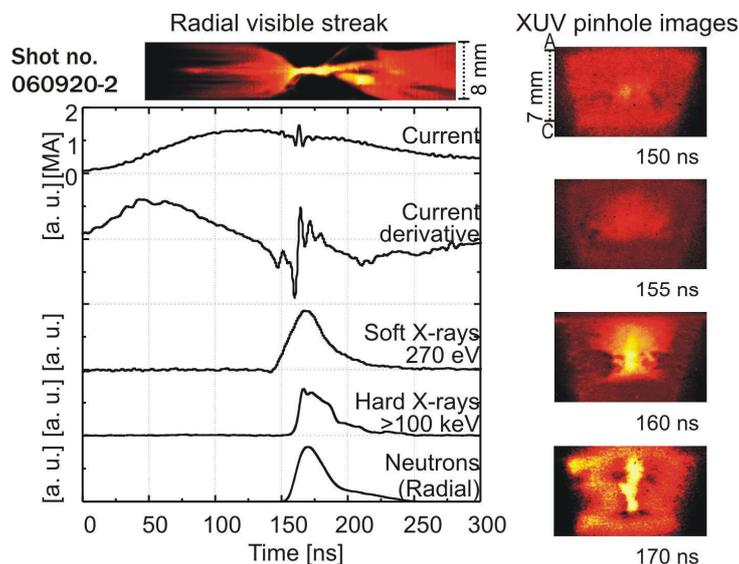
**Figure 1.** Waveforms of current, current derivative, X-ray and neutron emission together with XUV pinhole and streak images recorded in discharge no. 060920-2, neutron yield of  $4 \times 10^8$ .
