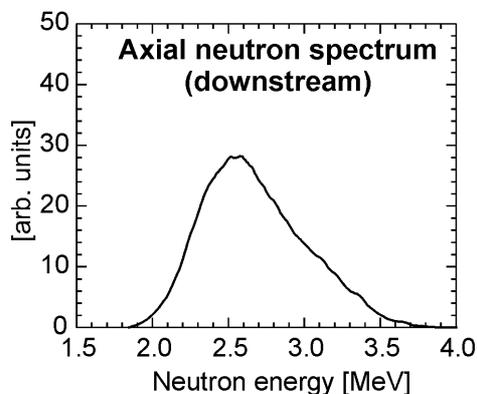
**Figure 2.** Axial neutron energy spectrum emitted in shot no. 060920-2, neutron yield of  $4 \times 10^8$ .
