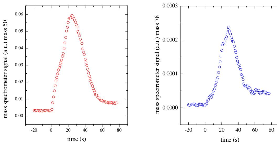
Figure 2: Left view graph: mass spectrometer signal for mass 50 as a function of time. The onset of dust formation occurs at about  $t = 20$  s. Right view graph: mass spectrometer signal for mass 78 as a function of time.
