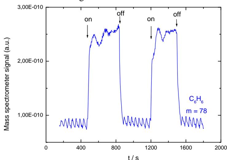
Figure 4: Mass spectrometer signal for mass 78 (benzene) The vertical arrows indicate the time when the second discharge is switched on and off respectively.
