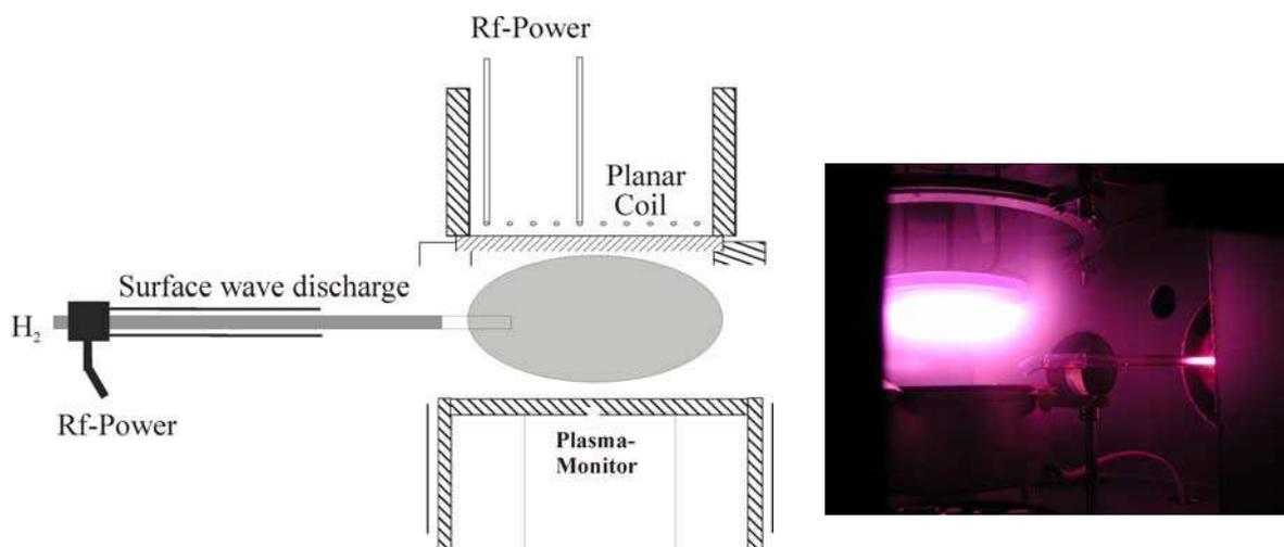
Figure 3: Sketch of the double plasma experiment. The double plasma experiment consists of two parts: the main plasma chamber with the inductively coupled discharge and the surface wave produced plasma running in a glass cylinder that reaches out into the main chamber. The second discharge - that is operated with hydrogen - is used to enhance the amount of atomic hydrogen that flows into the main chamber.
