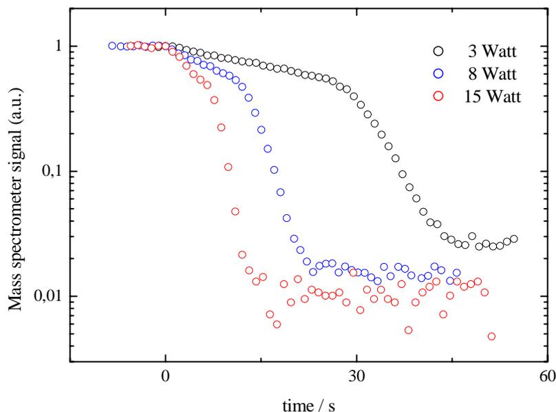
Figure 1: Mass spectrometer signal for mass 26 (acetylene) as a function of time. capacitively coupled discharge operated in a mixture of argon (8 sccm) and acetylene (0.5 sccm).
