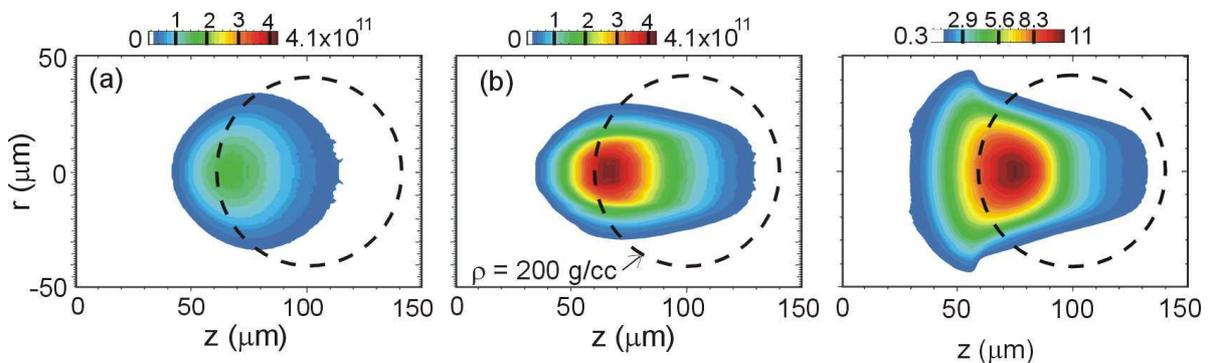
**FIG. 3.** Comparison of the energy density (in  $\text{J/cm}^3$ ) deposited by the fast electron beam with an initial divergence of  $22^\circ$  (FWHM): (a) simulation with self-generated fields artificially suppressed and (b) full simulation. (c) Ion temperature distribution in keV at the end of the pulse in the case (b). Dashed circles show the initial density contour of  $200 \text{ g/cm}^3$ .
