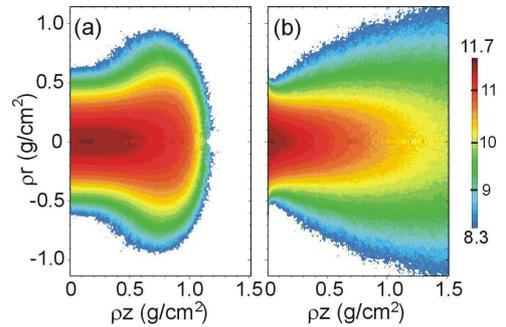
**FIG. 2.** Energy deposition isocontours of (a) 2.2 MeV electrons impinging perpendicularly on a DT slab and (b) electrons with a mean energy of 2.2 MeV and a divergence angle of  $22^\circ$ .
