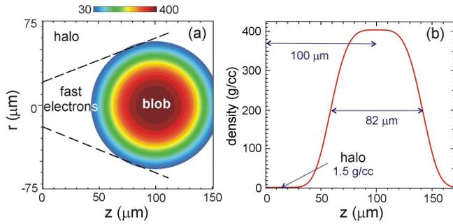
**FIG. 1.** Central cut through imploded target configuration: (a) density isocontours in  $\text{g/cm}^3$  and (b) density profile at  $r = 0$ .
