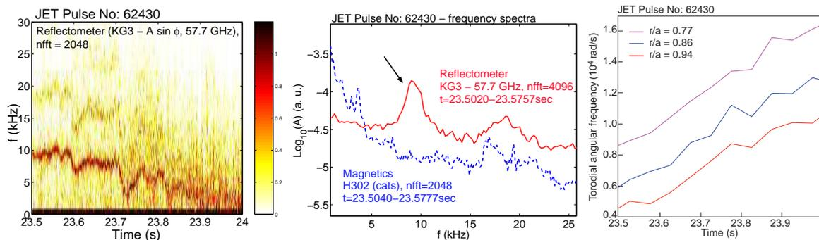
Figure 2: (a) Spectrogram from reflectometry showing narrowbanded density fluctuations, (b) comparison of frequency spectra from reflectometry and fast magnetics. The density fluctuations are not detected on the magnetic fluctuation signal. (c) Time evolution of the edge plasma rotation, obtained by charge exchange recombination spectroscopy.
