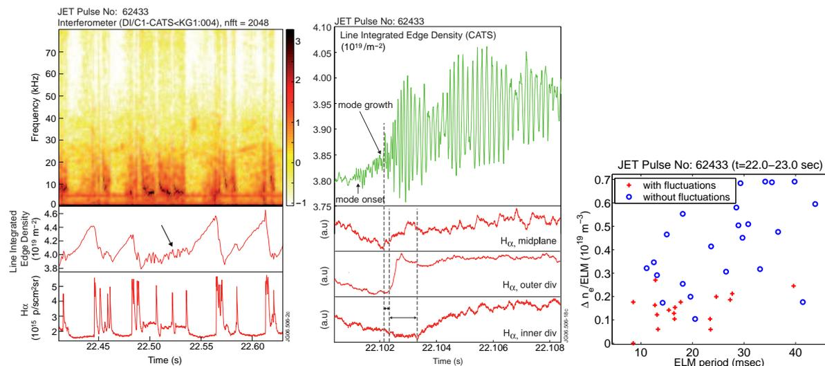
Figure 4: (a) Spectrogram of the edge chord signal of the FIR interferometer, showing isolated phases with density fluctuations between some type-I ELMs. Also shown are the line-integrated edge density and the H<sub>α</sub> emission in the outer divertor. (b) Timings for onset of enhanced emission at various locations (c) comparison of ELM-induced particle losses for ELM periods with and without the density fluctuations
