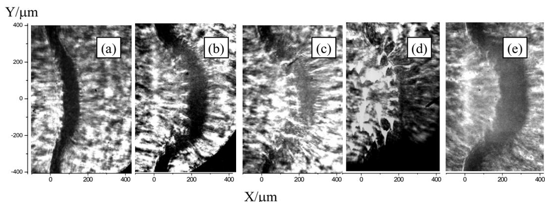
Figure 3. Temporal evolution of the RT instability. (a)  $\Delta t=-1050$ ps, the spikes and bubbles were not clear. (b)  $\Delta t=-650$ , (c)  $\Delta t=-250$ ps, (d)  $\Delta t=0$ ps, they developed. (e)  $\Delta t=150$ ps, the spikes and bubbles mixed.
