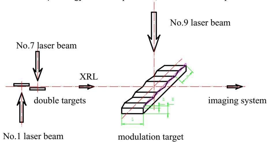
Figure 1. Experimental setup. Two laser beams (No.1 and No.7 laser beam) were employed to create the XRL. The RT instability plasma was produced by irradiating the No.9 laser beam onto a modulation target.
