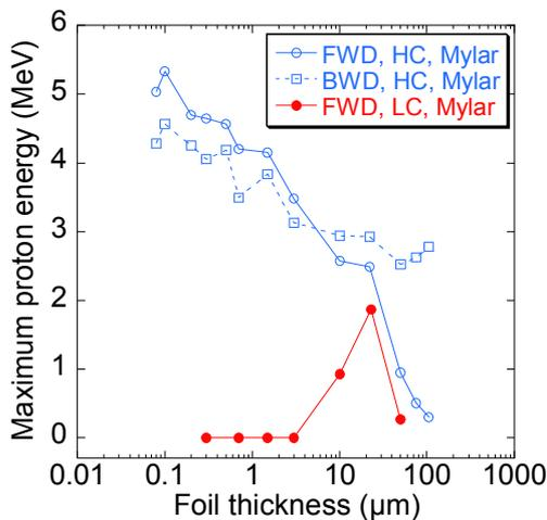
Figure 2 : Variation of maximum proton energy as a function of target thickness of FWD and BWD emission for laser contrast of  $10^{10}$  ( $510^{18}$  W/cm<sup>2</sup>) and  $10^6$  ( $10^{19}$  W/cm<sup>2</sup>)
