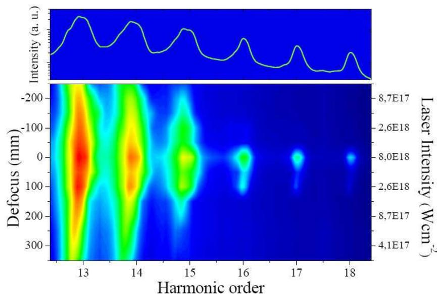
*Figure 1 : Harmonic spectrum dependency on the laser intensity. Harmonic spectra obtained on plastic are plotted in logarithmic scale as a function of distance between the target surface and the laser best focus.*
