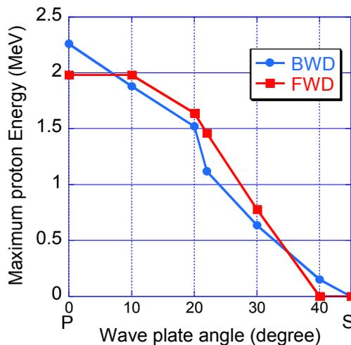
Figure 3: Variation of maximum proton energies as a function of laser polarization in the HC case.
