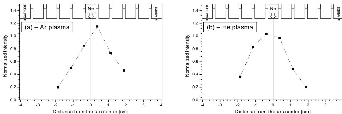
Fig.2. Axial distributions of Ne I 692.9 nm intensities, obtained by integration along the arc diameter. The values have been divided by the intensity corresponding to the position of neon injection.
