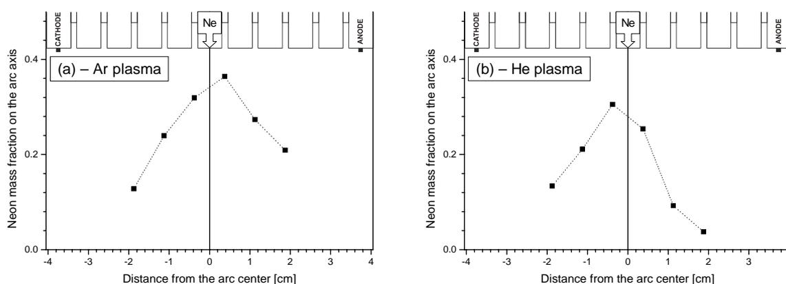
Fig.4. Axial distributions of neon mass fraction values on the arc axis are shown.
