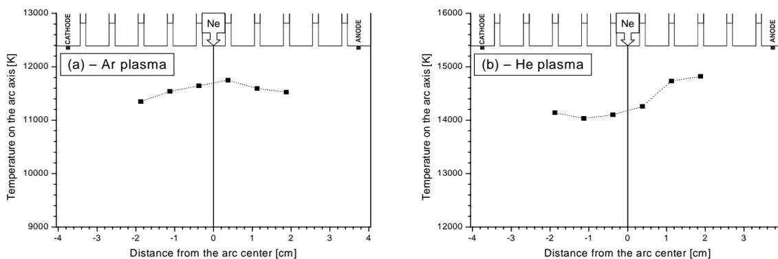
Fig.3. Axial distributions of temperature values on the arc axis are shown .
