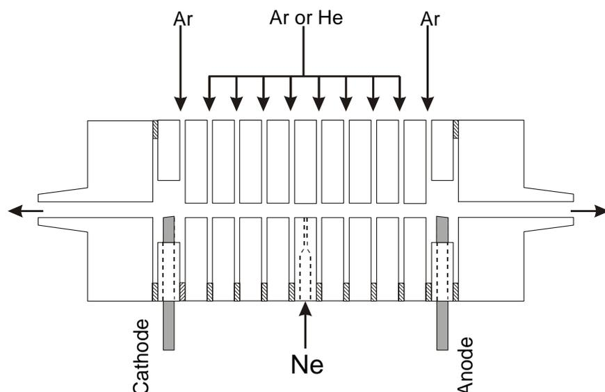
Figure 1. The scheme of the arc construction and the gas flow system is shown.
