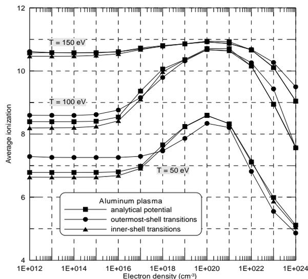
Fig. 1. Influence of energy levels structure on average ionization. Calculations were done for an aluminum plasma.
