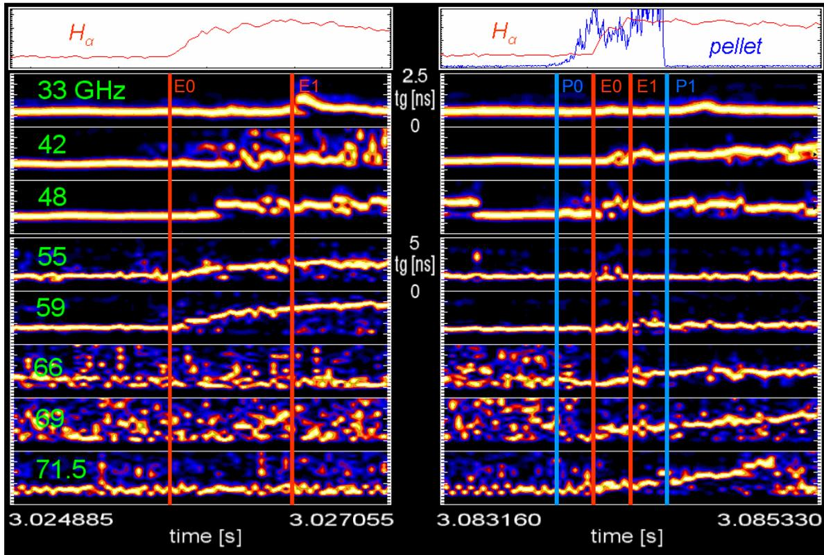
69 GHz ( $n_e=5.9 \cdot 10^{-19} \text{ m}^{-3}$ ) and 71.5 GHz ( $n_e=6.4 \cdot 10^{-19} \text{ m}^{-3}$ ) the reflected signal cannot be detected because the density is not sufficiently high to reflect the probing microwaves. At 71.5 GHz the detected spectrum corresponds to the noise base line of the heterodyne detection. In the case of the pellet triggered ELM, we first notice that the movements of the
