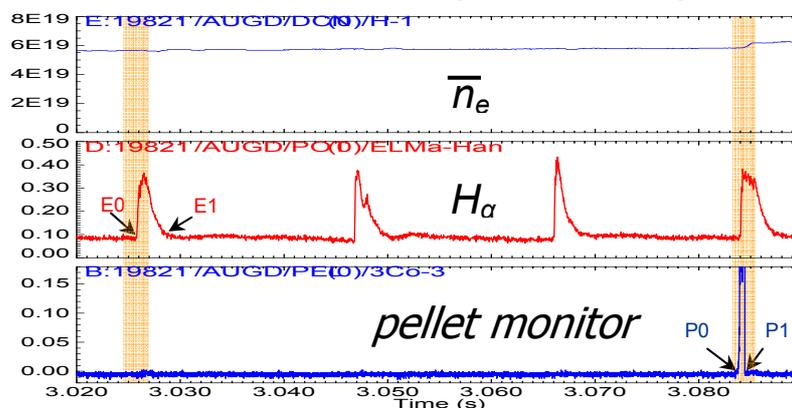
flux indicated by the peak of the  $H_\alpha$  signal. For this reason we developed a new method to visualize in a simple and direct way the local profile changes, without the need to evaluate the density profile. The method uses the spectrogram of the plasma reflected signals derived from swept frequency data (basic information for density profile inversion) and
