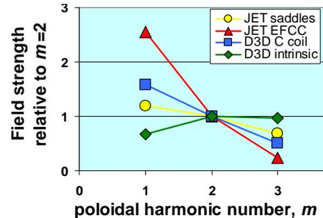
Fig 5: Error field spectra on JET and DIII-D.
