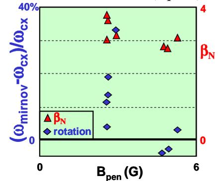
Fig 4: DIII-D rotation in ExB frame falls as error field rises and rotating 2/1 NTM threshold falls.
