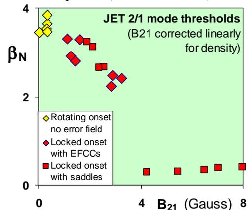
Fig 2: JET error field thresholds at various constant heating powers.
