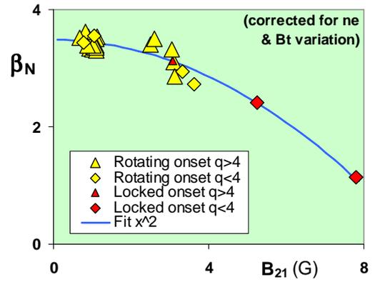
Fig 3: DIII-D 2/1 NTM  $\beta_N$  threshold as a function of error field applied.
