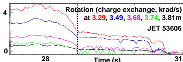
Fig 6: Locking of  $q=2$  surface (3.71m, 28.7s) by JET saddle coils while core plasma still rotates.
