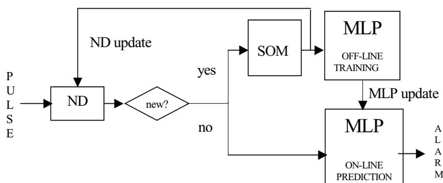
Figure 1 Disruption prediction scheme – on line application
