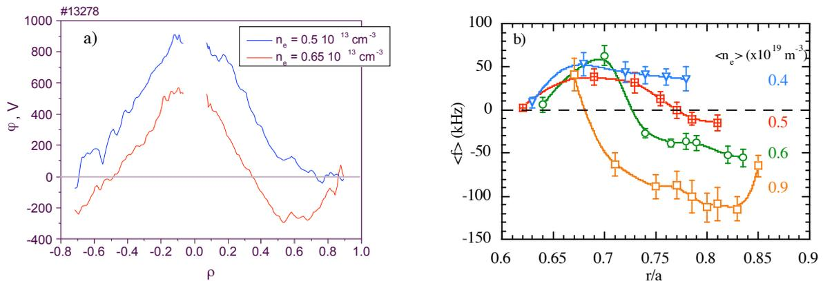
Fig. 3.- a) Plasma potential measured by HIBP at two plasma density values. b) Mean frequency of the spectra vs. cut-off radius increasing density.
