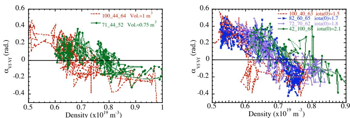
Fig. 4.- Plasma volume and iota effects on the threshold density value. Figure shows the phase between two floating potential signals poloidally separated 0.3 cm for different plasma density values. Measurements were taken at the plasma edge ( $r/a \approx 0.85-1$ ). Lines are guides for the eye.
