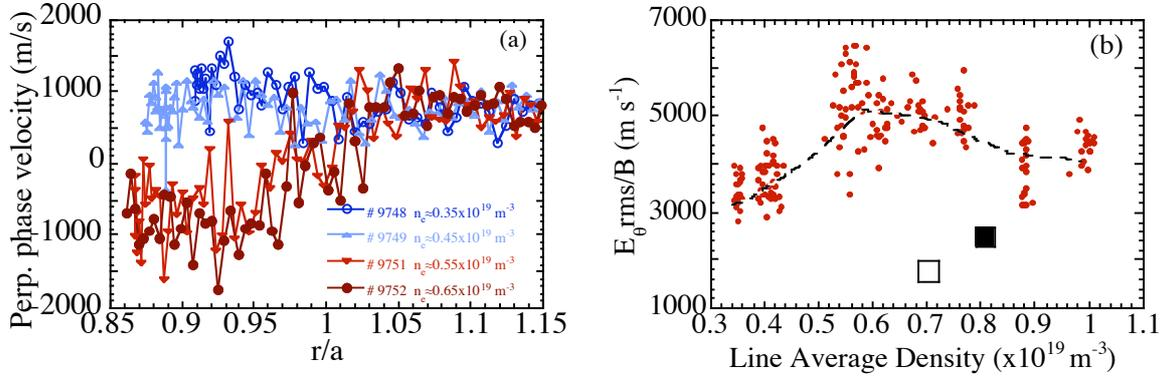
Fig.1- (a) Radial profiles of the perpendicular phase velocity for different plasma density. (b) Behaviour of the perpendicular radial velocity as a function of the density. The open square corresponds to biasing experiment and closed one to naturally obtained improved confinement regime results (see section 4). Line is a guide for the eye.
