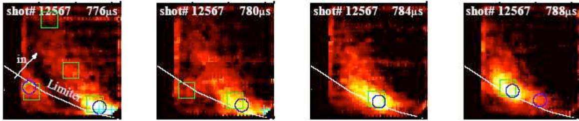
Fig. 2.- Poloidal movement and position of located blobs (big scale-green squares, medium scale-blue circles, small scale-light blue pluses).
