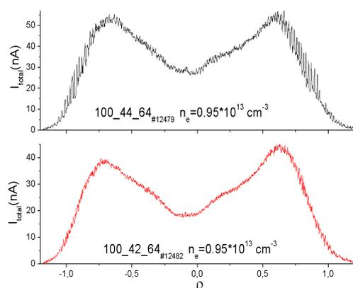
**Fig.1** Cs<sup>2+</sup> current (electron density) profiles versus magnetic configuration
