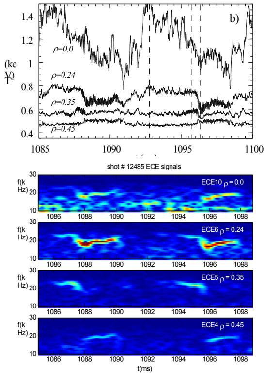
**Fig. 3.** Time evolution of the electron temperature (ECE) in a plasma with e-ITB formation at 1092 – 1095 ms. Lower boxes – time evolution of the  $T_e$  frequency spectra for various  $\rho$ .
