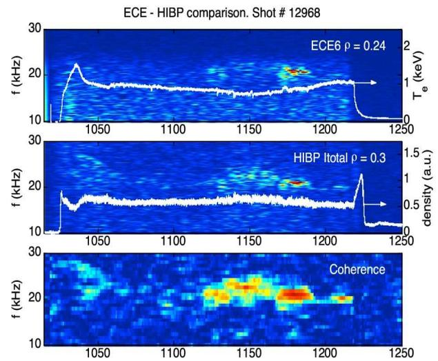
**Fig. 4.** Comparison HIBP and ECE signals: (a) ECE evolution and spectrum at  $\rho \approx 0.24$ , (b) HIBP  $Cs^{2+}$  current and spectrum at  $\rho \approx 0.3$  (c) coherence between them.
