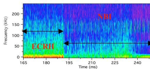
Figure 4. Power spectrum of ion saturation current fluctuations for ECRH and NBI plasma phases in the scrape-off layer region.
