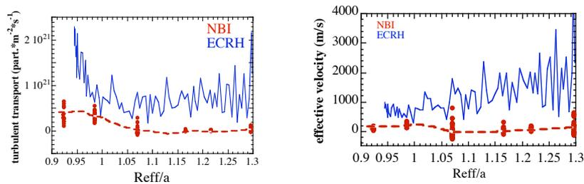
Figure 2. Scanning of NBI plasma shots showing the ExB turbulent driven flux and radial effective velocity of events spreading radially outward.
