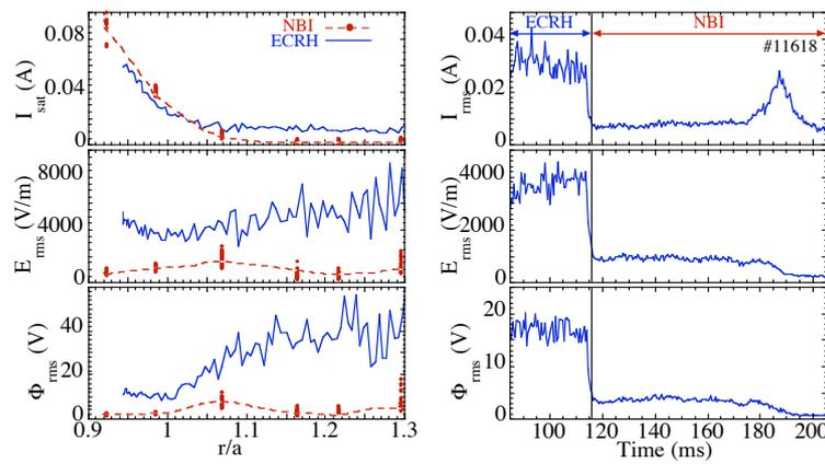
Fig. 3 LE Figure 1. LEFT: Radial profiles measured in the ECRH and NBI plasmas. Measurements in NBI plasmas were taken shot to shot at a plasma density of about  $3 \times 10^{19} \text{ m}^{-3}$ , RIGHT: the time evolution of the edge level of the fluctuations during the transition from ECRH to NBI.
