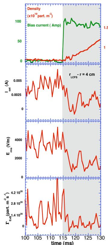
Figure 5. Time evolution of the main parameters for a discharge with DC electrode biasing ( $V_{\text{bias}} = -300\text{V}$ ). The shadowed area indicates the time when the bias is applied
