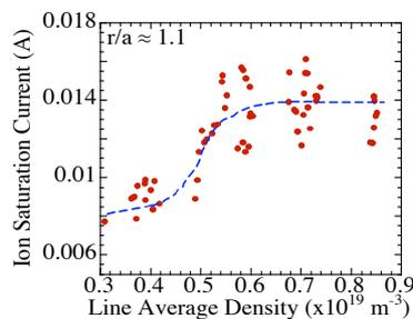
Figure 3. Ion saturation current as a function of the plasma density measured in the scrape-off layer.
