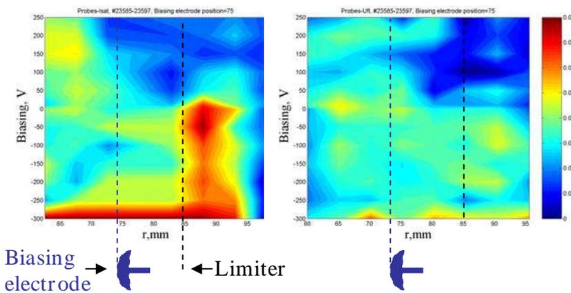
Fig. 2 Rake probe / bias. voltage,  $I_{sat}$  (left) and  $U_{fl}$  (right)
