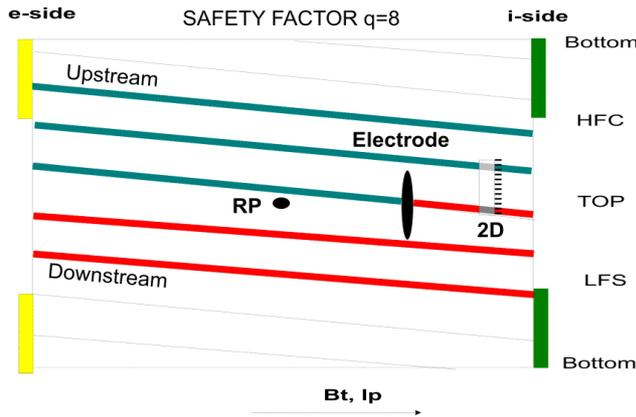
**Fig 1.** Unfolded magnetic surface: The surface is cut at the limiter and the bottom. Toroidal and poloidal position of the probe arrays and of the electrode is marked. The flux tube emanating from the electrode either upstream or downstream along the magnetic field line is emphasized by different color.
