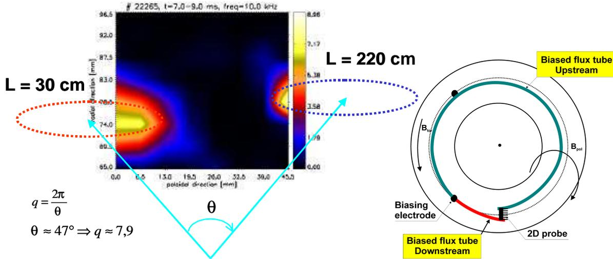
**Fig. 3** Left: Power spectra from the 2D probe with parallel set-up. Right: Trace of the flux tube associated with the electrode.
