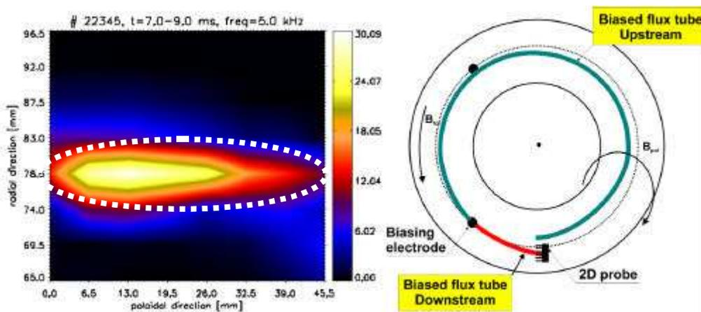
**Fig. 2** Left: Power spectra from the 2D probe with antiparallel orientation. Right: Trace of the flux tube associated with the electrode.
