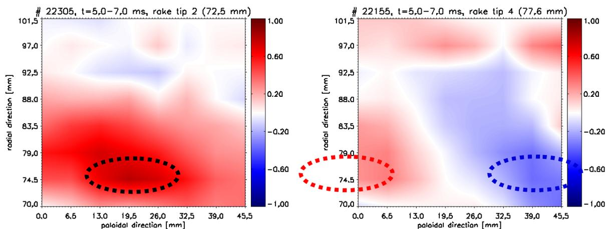
**Fig. 4** Cross-correlation functions of a rake probe tip with the 2D probe matrix. Left: Rake probe tip 2 (72.5 mm radially from the centum of plasma), antiparallel orientation. Right: Cross-correlation functions of the rake probe tip 4 (77.6 mm) with 2D probe matrix, parallel orientation.
