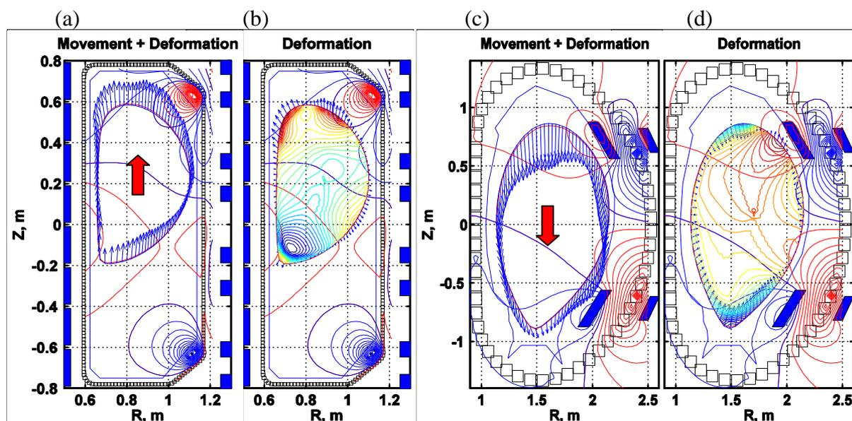
**Figure 2.** The third candidate, the flux surface deformation patterns. ELMs are triggered. (a) and (c) : plasma movements and the flux surface deformation in TCV and ASDEX Upgrade, respectively. (b) and (d) : the flux surface deformation in TCV and ASDEX Upgrade, respectively. All arrows are amplified by 20 times to make them visible.
