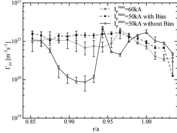
Fig. 3. Radial profiles of the particle flux  $\Gamma_{es}$  due to the electrostatic fluctuation with plasma biasing (solid line), without plasma biasing (dashed line) and  $I_p^{\max} \approx 60$  kA (dotted line).
