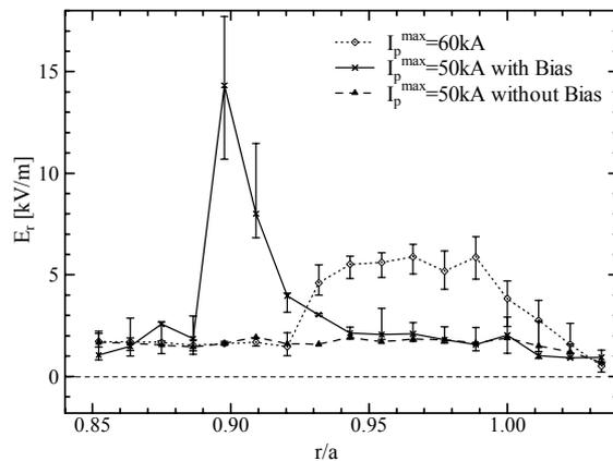
Fig. 2. The radial electric field  $E_r$  profiles with plasma biasing (solid line), without plasma biasing (dashed line) and  $I_p^{\max} \approx 60$  kA (dotted line).
