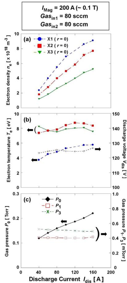
Fig. 4 Dependence of discharge current  $I_{dis}$  for (a) central density of each probes, (b) electron temperature  $T_e$  and discharge voltage  $V_{dis}$  and (c) gas pressure at each vacuum gauge.
