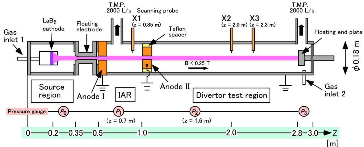
Fig. 1 Schematics of NAGDIS-II with two anode of Anode-I and Anode-II.
