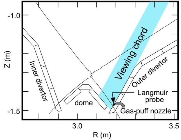
Figure 1: *Cross-sectional view around the divertor. Viewing chord for the spectroscopic measurement, location of the gas-puff nozzle, and the magnetic configuration are shown. Another viewing chord and a Langmuir probe are positioned on different poloidal cross-sections.*
