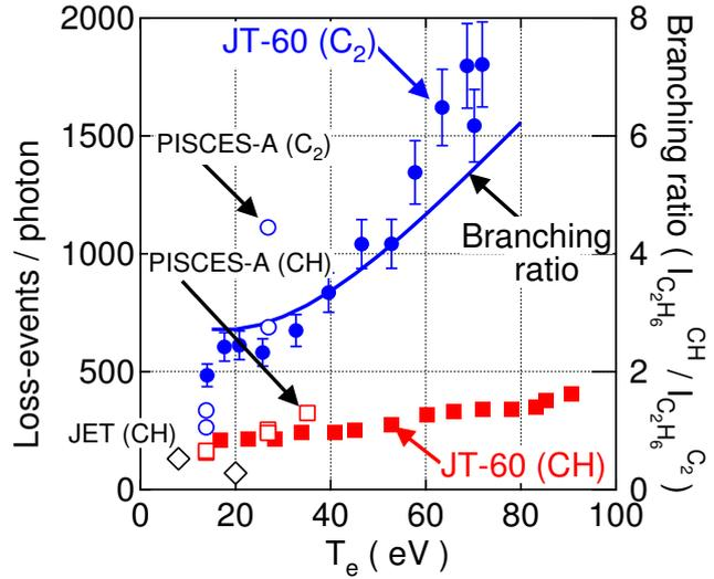
Figure 4: Loss-Events / Photon ( $LEP_{C_2H_6}^{CH}$  and  $LEP_{C_2H_6}^{C_2}$ ) and branching ratio,  $B_{C_2H_6}$ , as a function of electron temperature. Data taken for  $C_2H_4$  in PISCES-A [6] (open circles for  $C_2$  and open squares for CH) and JET [9] (open diamonds) are also shown.
