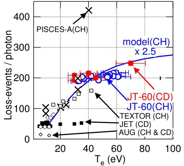
Figure 3: Loss-Events / Photon ( $LEP_{\text{CH}_4}^{\text{CH}}$  and  $LEP_{\text{CD}_4}^{\text{CD}}$ ) as a function of electron temperature (electron density:  $0.5 - 2 \times 10^{19} \text{m}^{-3}$ ). Data taken in JET [3] (closed squares), AUG [4, 5] (open diamonds), PISCES-A [6] (crosses), TEXTOR [7] (open squares), and data from model calculation [8] (solid curve) are also shown.
