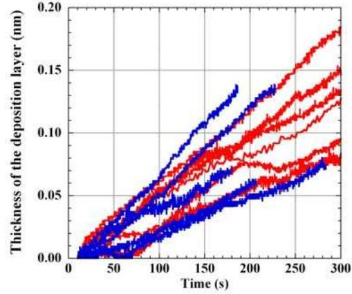
*Fig.4 Growth of the deposition layer of Mo on the viewing window of sapphire during the long duration discharges. Red and blue lines indicate the discharges with and without the ML, respectively.*
