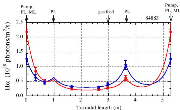
Fig.5 Toroidal profiles of the  $H_{\alpha}$  intensity before (red) and after (blue) the drawing up of the ML.
