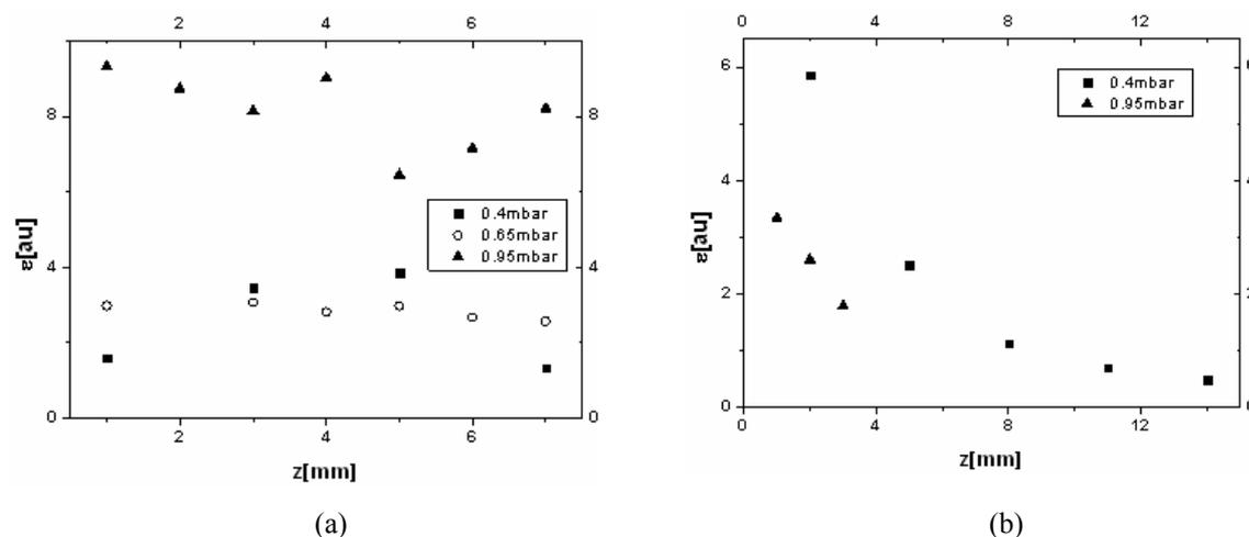
Fig.3. Plasma emissivity along the axis of symmetry for different pressure values:
