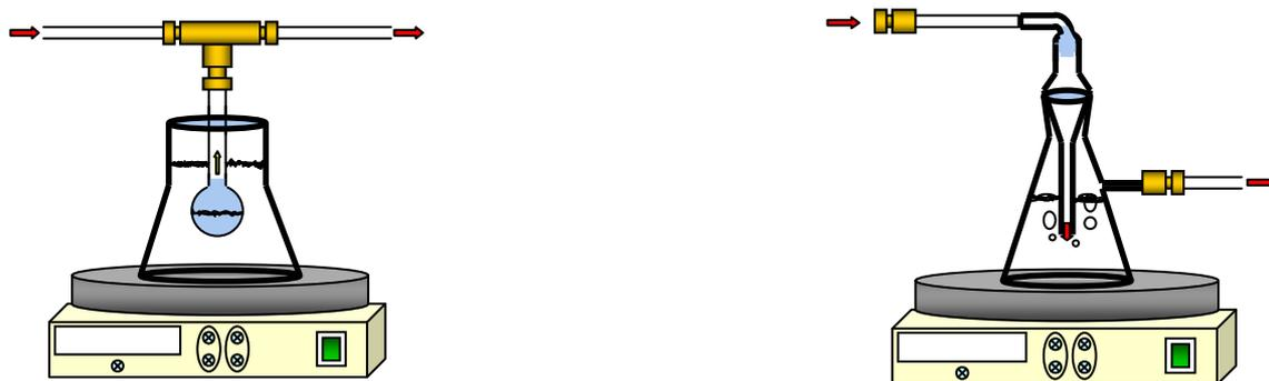
**Figure 2.** *Sweeping (left) and bubbling (right) sample introduction arrangements.*
