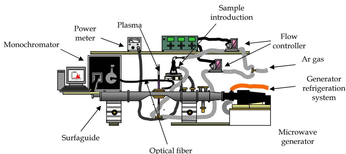
**Figure 1.** Diagram of the experimental arrangement
