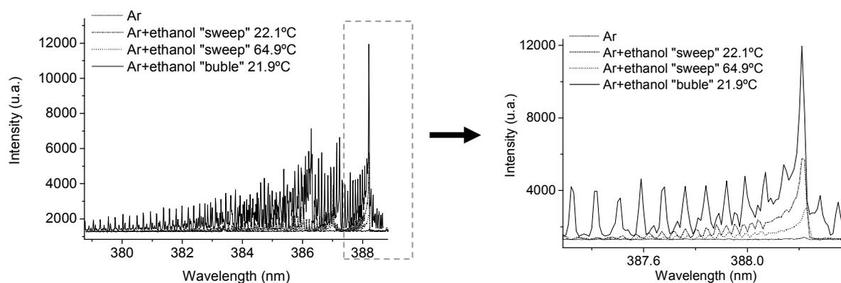
**Figure 3.** *CN rotational band (left) for different introduction methods and experimental conditions and detail on band head (right)*
