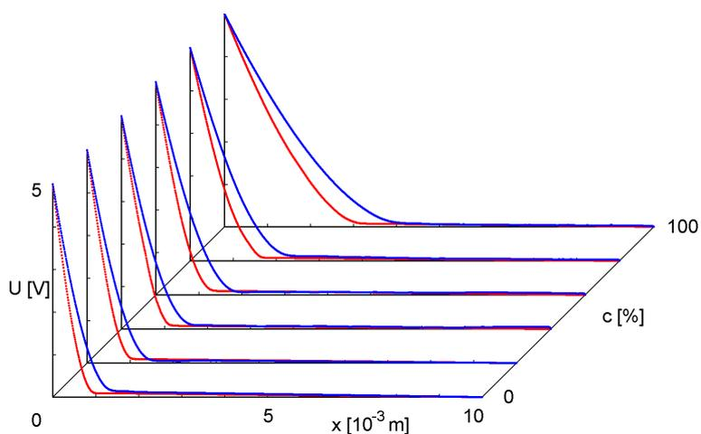
Figure 2: Potential distributions  $U(x)$  in the sheath for various relative concentrations of negative ions  $c$ . Pressure of plasma: blue – 133 Pa, red – 1330 Pa. Planar geometry.
