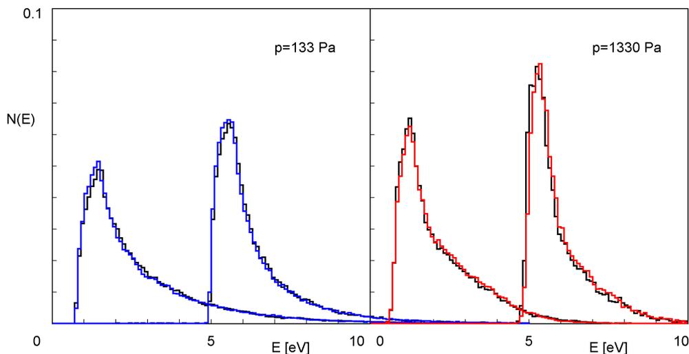
Figure 3: Energy distributions of electrons at two plasma pressures, both in two positions in the sheath – on the boundary sheath-presheath (left characteristics) and on the surface of immersed solid (right). Planar geometry, applied voltage bias +5 volts. Original electron temperature 2 eV.
