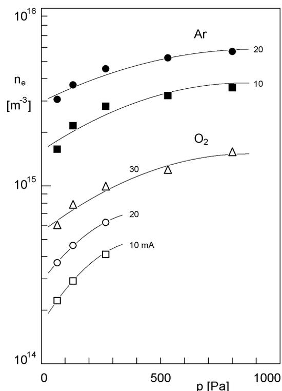
Figure 1: Electron densities in positive column of dc glow discharge in argon and oxygen. Discharge current 10 to 30 mA.
