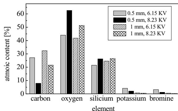
Fig. 6 Atomic content of O, Si, C, K and Br of coatings on KBr deposited in HMDSO-Ar-O<sub>2</sub> (33 vol.-% O<sub>2</sub>) with different applied voltages
