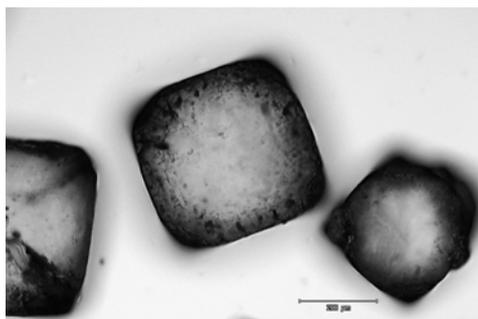
Fig. 2 NaCl particles coated in TEOS-Ar-O<sub>2</sub>
