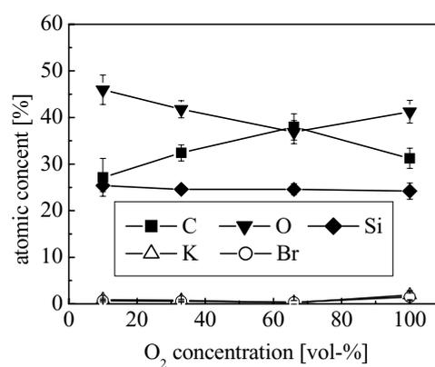
Fig. 5 Atomic content of O, Si, C, K and Br of coatings on KBr deposited in HMDSO-Ar-O<sub>2</sub> with different oxygen concentrations, thickness of dielectric barrier: 1 mm
