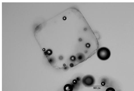
Fig. 3 Remaining coating after dissolution of NaCl crystal in water. The coating was deposited in TEOS-Ar-O<sub>2</sub>.
