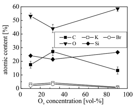
Fig. 4 Atomic content of O, Si, C, K and Br of coatings on KBr deposited in HMDSO-Ar-O<sub>2</sub> with different oxygen concentrations, thickness of dielectric barrier: 0.5 mm
