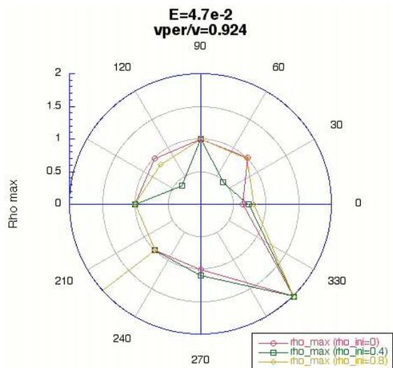
**Figure 1.** Polar plot of the maximum effective radius reached by particles of very low energy and high perpendicular velocity starting from different radius. The particle is considered to escape when it arrives at  $\rho=1$ .
