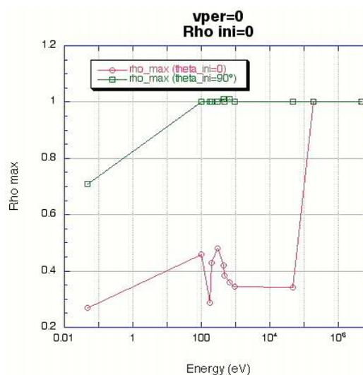
**Figure 2.** Maximum effective radius reached by particles with only parallel velocity and born in the centre of the plasma for two different poloidal angles.
