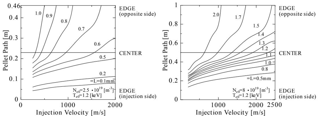
Fig 1(a). Typical results of the pellet penetration depth into JIPP T-IIU plasma as a function of the pellet velocity, where the pellet size is varied from 0.1 to 1.0mm
