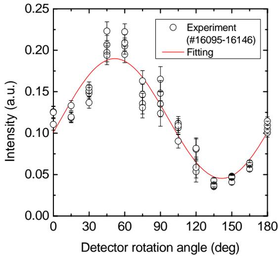
Fig. 3 Dependence of measured EC wave intensity on detector rotation angle
