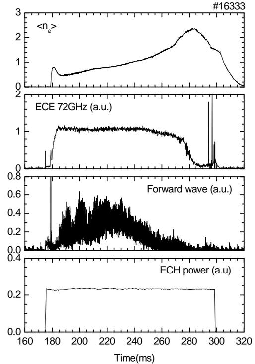
Fig. 1 Time evolution of ECH plasma in Heliotron J
