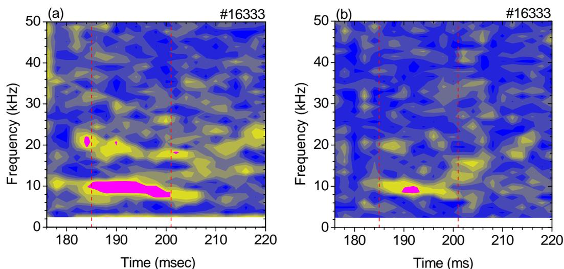
Fig. 5 Correlation of forwardly scattered EC waves with (a) core electron density and (b) magnetic fluctuation.
