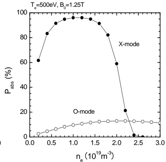
Fig. 4 Ray tracing calculation of single pass absorption rate
