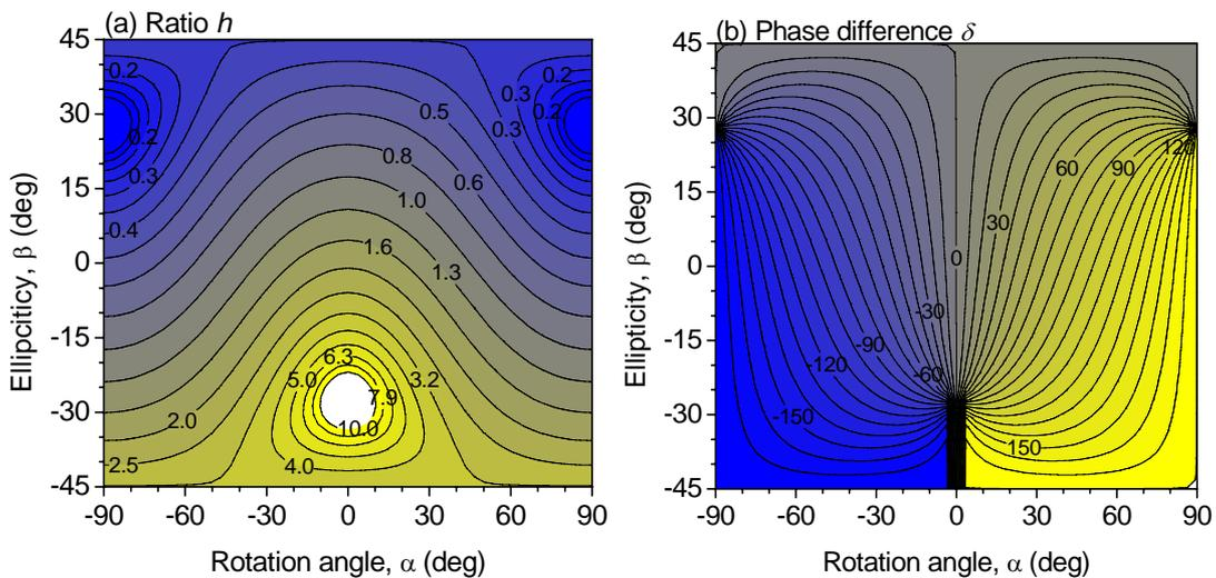
Fig. 2 Mode mixture of forward waves in Heliotron J, (a) ratio,  $h$  and (b) phase difference,  $\delta$
