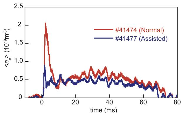
Fig.4 Time evolution of line-averaged electron density  $\langle n_e \rangle$ .
