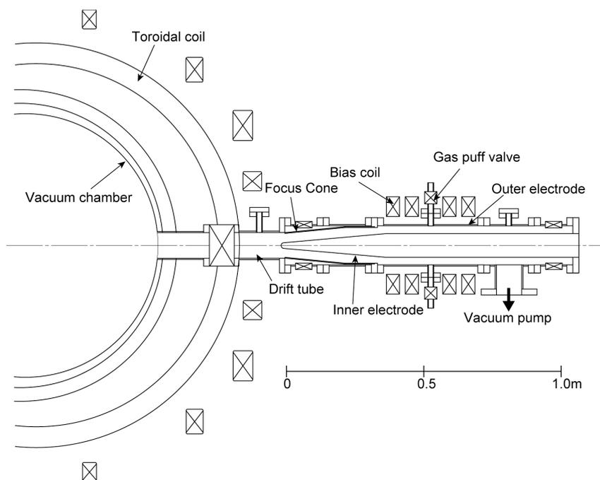
Fig. 1 Schematic view of a poloidal cross section (toroidal angle  $\phi = 225^\circ$ ) of TPE-RX device and a helicity injector.
