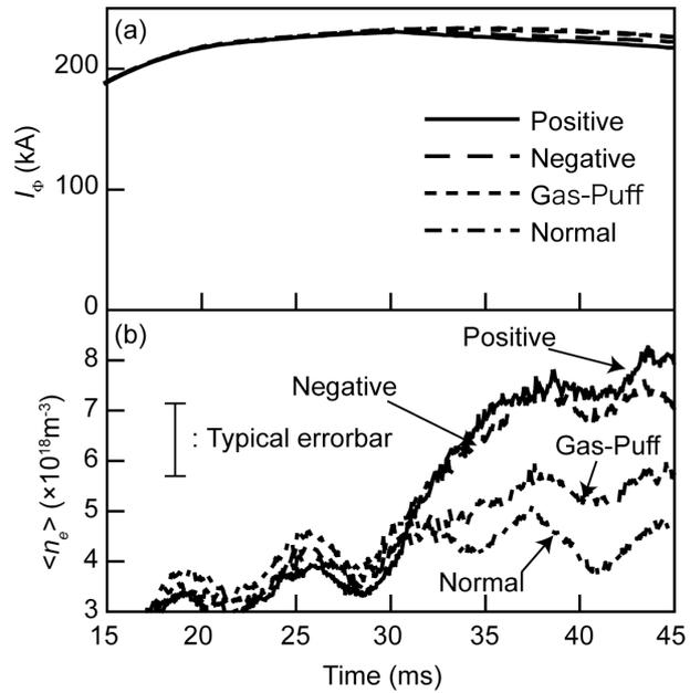
Fig. 2 Time evolution of (a) plasma current  $I_\phi$  and (b) line averaged electron density  $\langle n_e \rangle$  measured at  $\phi=135$ .
