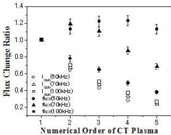
Fig. 4 Dependence of accumulation effect on repetition frequency
