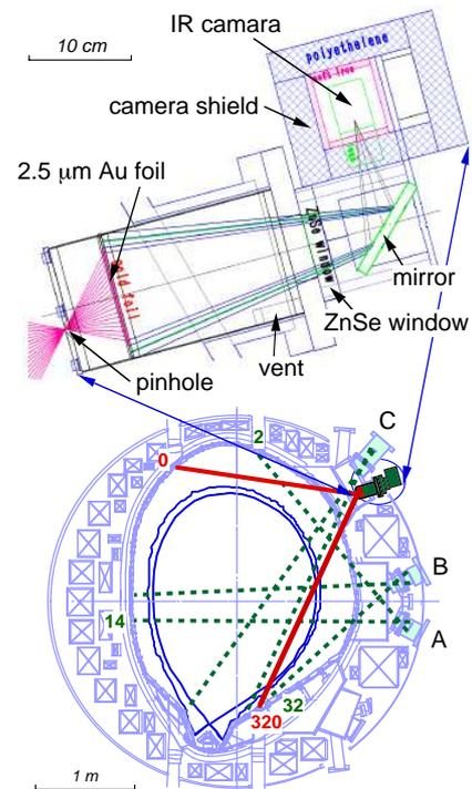
Fig. 1 IR imaging bolometer (top) and FOV in JT-60U (bottom thick lines), and resistive bolometer arrays, A-C (FOV, broken lines).
