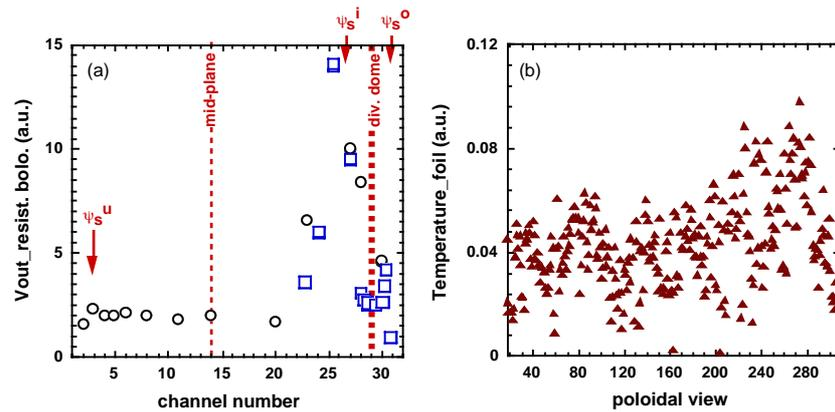
Fig. 5 Comparison of profiles by resistive bolometers, circles by A and B and squares by C arrays (a), and by imaging bolometer (b) at 15.5 sec. Channel numbers and picture pixels are shown in Fig. 1
