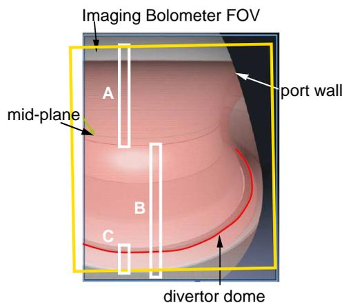
Fig. 2 3D FOV by a computer. A large rectangle is imaging bolometer view (brown), white rectangles are views of resistive bolometers A, B and C. JT-60U plasma is colored pink.
