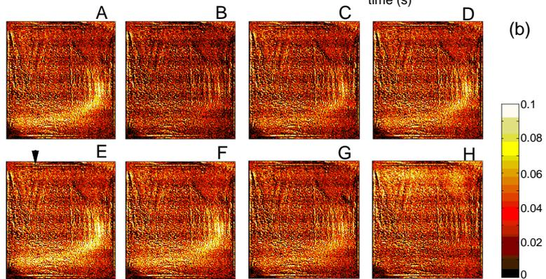
Fig. 4 (a) Time traces of a discharge and (b) 2D foil temperature images at A~H. Periodic horizontal lines in (b) are video signal aliasing artifacts.
