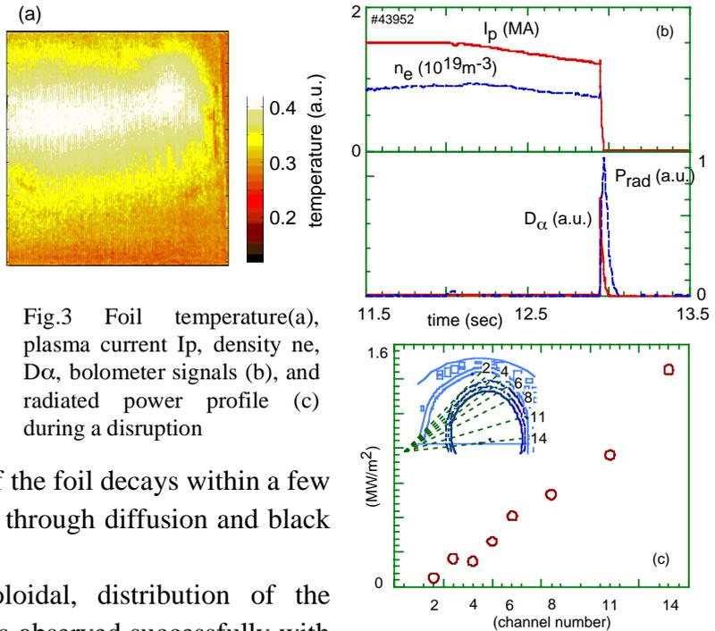
Fig.3 Foil temperature(a), plasma current  $I_p$ , density  $n_e$ ,  $D_\alpha$ , bolometer signals (b), and radiated power profile (c) during a disruption
