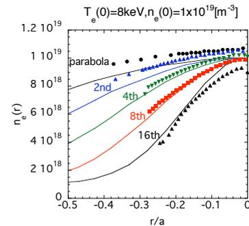
Fig.5.  $n_e(r)$  assumed (solid lines) and derived (solid marks).
